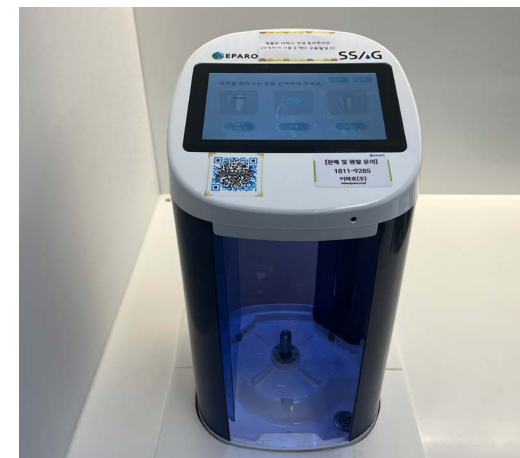
Automatic tumbler washing machine at ICT site
